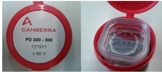
Figure 3.1: PIPS detector PD 300-300 of the company Canberra
